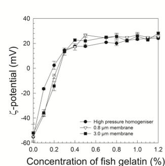
**Fig. 2.** Effect of concentrations (0 - 1.2%) of fish gelatin on the ζ-potential. ζ-potential goes from -55 mV for primary liposomes to 25 mV for secondary liposomes.
