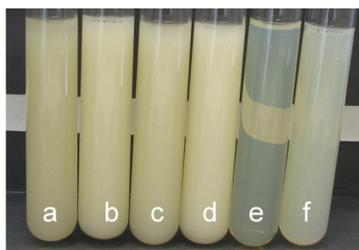
**Fig. 4.** (a) Primary and (b) secondary liposomal dispersions produced with extrusion through 3.0 µm membrane, (c) primary and (d) secondary liposomal dispersions produced with extrusion through 0.8 µm membrane and (e) primary and (f) secondary liposomal dispersions produced with high pressure homogenisation.
