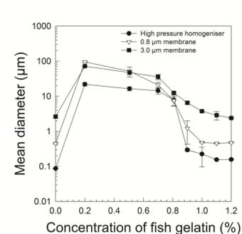
**Fig. 3.** Effect of concentration (0 - 1.2%) of fish gelatin on mean volume diameter ( $d_{4,3}$ ). A large mean diameter (0.1 - 1.0% fish gelatin) indicates bridging flocculation.
