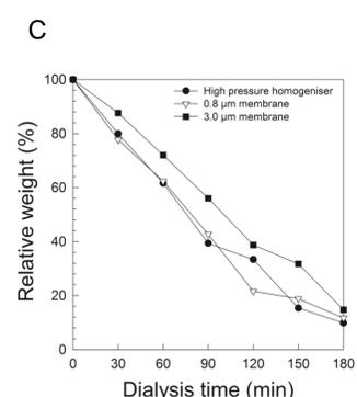
**Fig. 5.** Effect of dialysis time (0-180 min) with 0.5M sugar 10 mM acetate pH 3.8 on (A) relative weight ( $w_1/w_0$ ) and (B) mean volume diameter ( $d_{4,3}$ ) of primary liposomes and (C) relative weight and (D) mean volume diameter of secondary liposomes.
